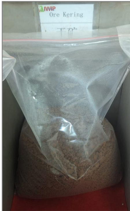
Figure 2. A sample of laterite ore from which nickel metal will be extracted.
