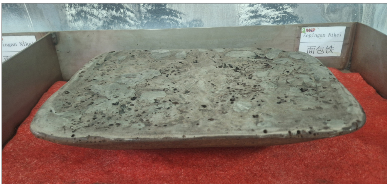
Figure 5. This photograph shows a sample of ferronickel obtained from the furnace
