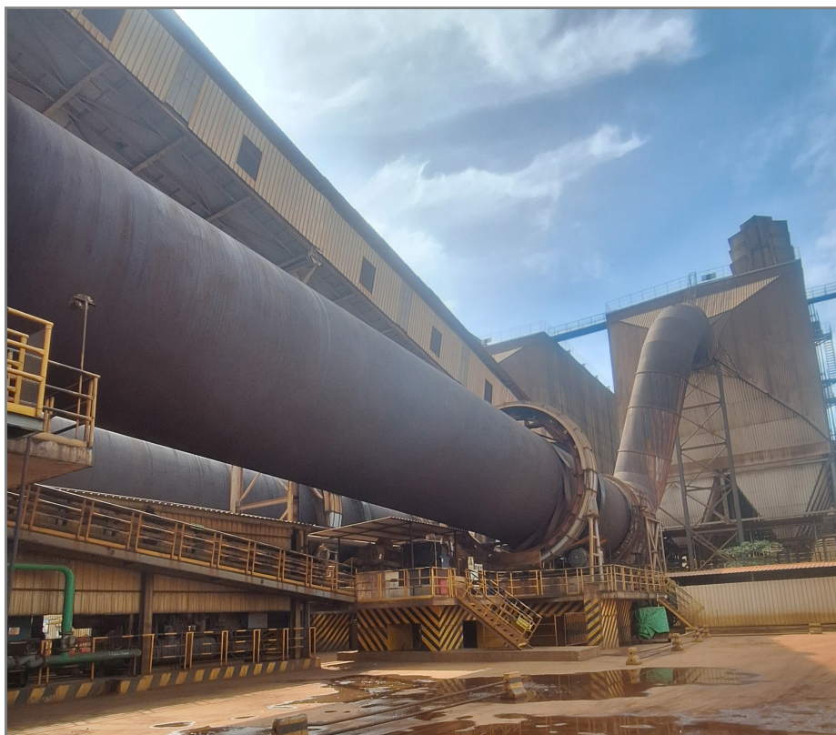
Figure 3 This photograph shows a drying kiln used to remove moisture from the ore.
